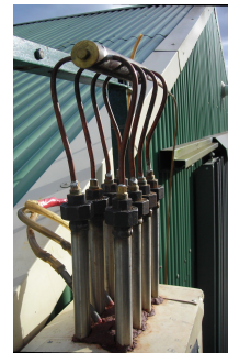
Figure 2. Two-plate, 8-tube ECP's FT test reactor of 5.5-L active catalyst volume (upper manifold).
