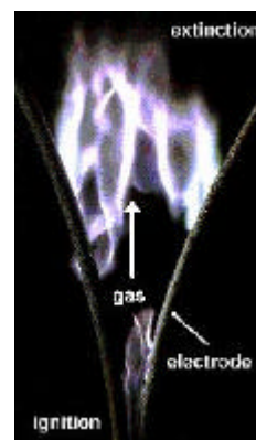
Fig. 1. Principle and time-integrated photo of the GlidArc-I discharge
