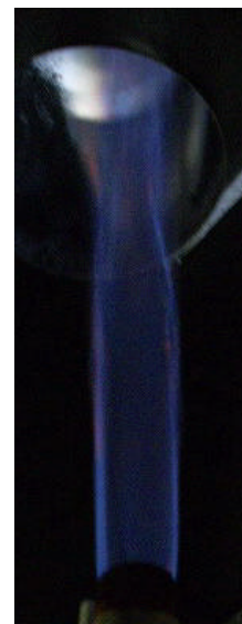
Fig. 7. Clean and soot-free syngas flare (diameter of 1.5inch)
